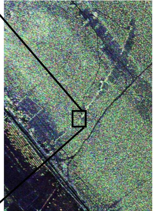
Fig.13: Geocoded E-SAR L-band SLC data in Pauli decomposition. Flight direction was approximately from upper right to lower left corner.
