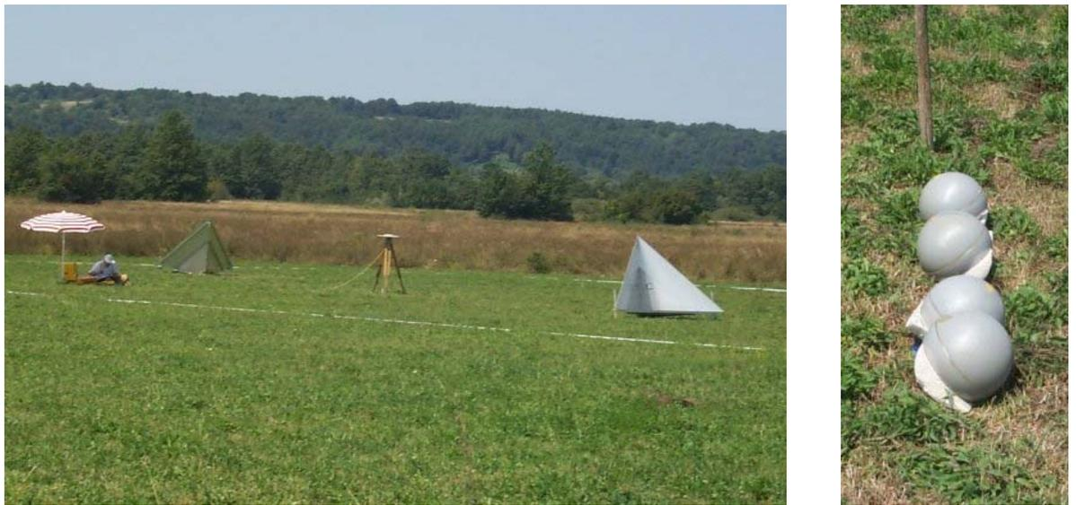
Figure 5: Ground team at the flight campaign in Glinska Poljana. Left image: Corner reflectors, GPS-system. Right image: Luneberg lenses at one position, looking into opposite directions.
