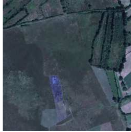
Figure 17. E-SAR P-band interferometric coherence of an agricultural used area and surrounding mine suspected fields in the Glinska Poljana test site. red: hhhh-coherence, green: xxxx-coherence, blue: vvvv-coherence
