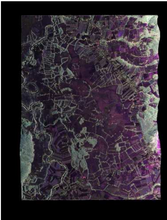
Figure 3. RGB-composite of geocoded E-SAR L-band images of Glinska Poljana (r,g,b = Lhh, Lhv, Lvv)
