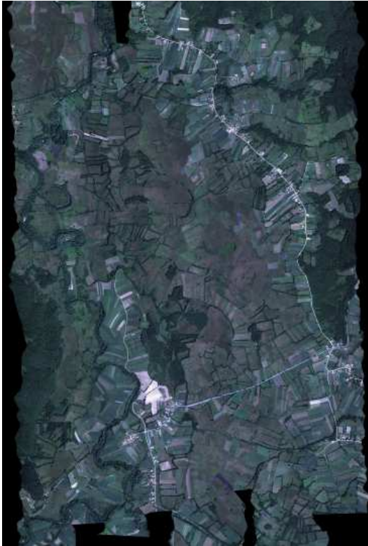
Figure 5. RGB-composite of geocoded Daedalus channels of Glinska Poljana. r,g,b = ch5 (red), ch3 (green), ch2(blue)
