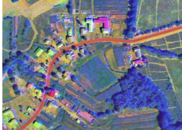
Figure 21. RGB composite of Daedalus and E-SAR geocoded data, village of Marinbrod. r,g,b: Daedalus ch11, ch9, E-SAR Lvv
