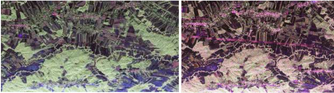
Figure 10. E-SAR L- and P-band images of Blinjski Kut in Pauli decomposition. red: even number of reflections, green: volume scattering and 45° tilted double bounce, blue: odd number of reflections
